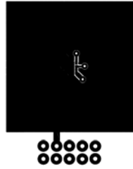
b. 50\text{ }^\circ\text{C/W} when mounted on a 1\text{ in}^2 pad of 2 oz copper
