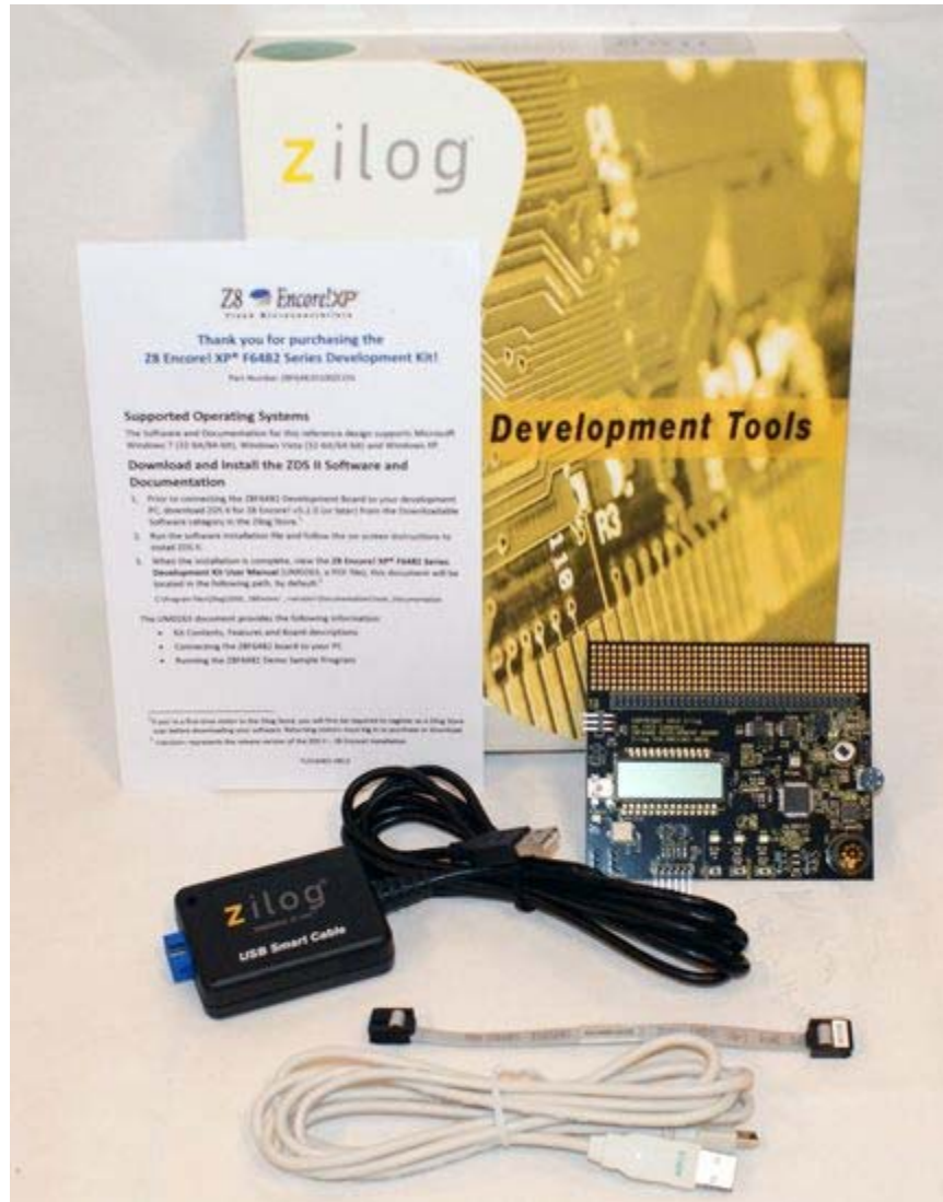
Figure 1. The F6482 Series Development Kit
