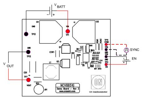
Figure 3. Evaluation Board Connections
