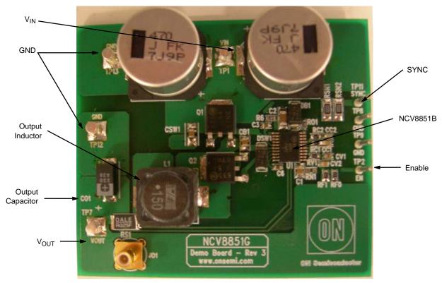
Figure 1. NCV8851B Evaluation Board
