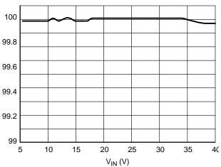
Figure 13. Line Regulation at 170 kHz, 13.2 V to 5 V Output
