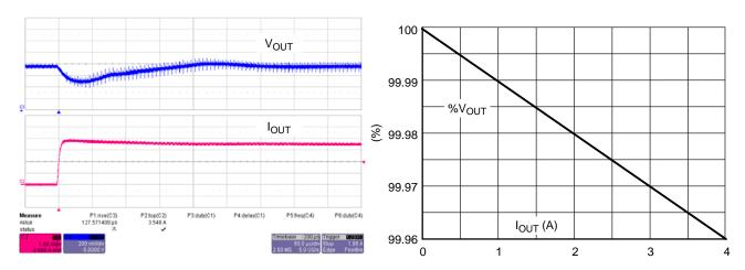
Figure 10. 100 mA to 3.6 A Load Step, 170 kHz, 5 V Output
