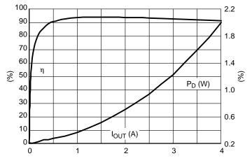
Figure 12. Efficiency at 170 kHz, 13.2 V to 5 V Output
