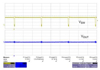
Figure 6. Minimum Duty Cycle at 170 kHz, 5 V Output
