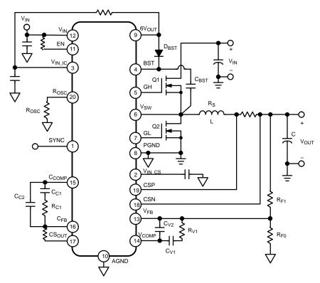
Figure 2. NCV8851B Application Diagram
